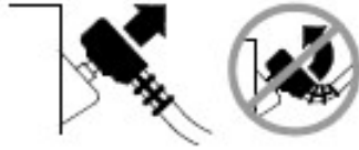
Figure 5-7 Disconnecting Defibrillation Cable from Test Post
