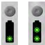
Figure 3-11 Battery Warning Indicators
